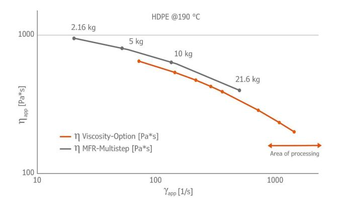
Using the mi40 visco with the L/D=10/1 mm die, is possible to measure materials with an apparent viscosity of 285 Pa\*s at apparent shear rate of 1000 1/s. The viscosity at a shear rate of 1000 1/s is quite common quality control criterion and available on a number of spec sheets. For a wide variety of materials, the mi40 visco is able to test at these conditions.
