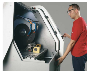
Two Hand Control For Safety Operation
