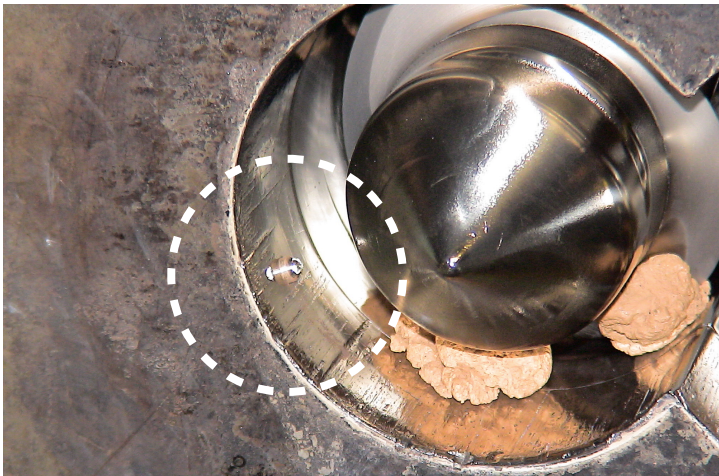
PHOTO 3. RPMP INSTALLED IN EXTRUDER
